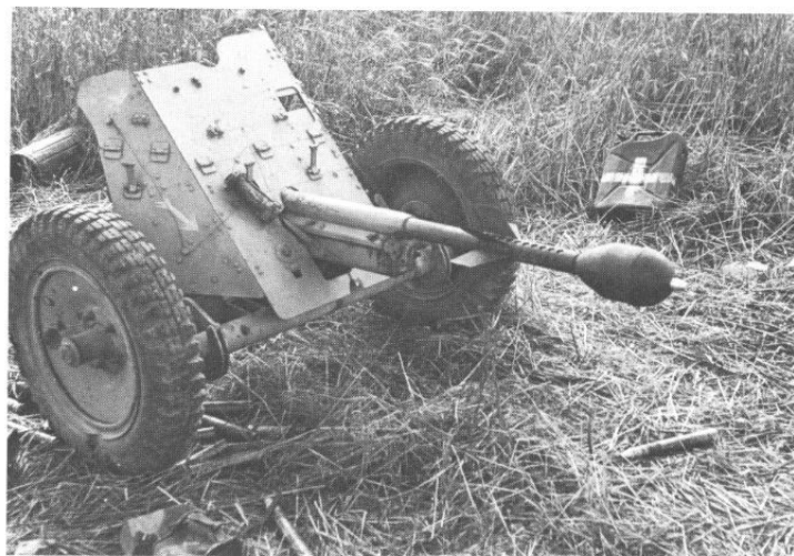
Pak 35/36 with the 3.7 cm Stielgranate 41. This was a hollow charge spigot grenade.
