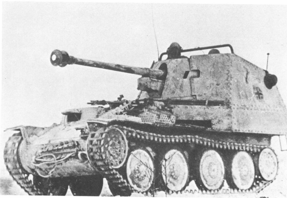
The Marder III Ausf M SdKfz 138 had its engine mounted forward and its 7.5 cm Pak 40 aft. This necessitated a special drivers compartment and new upperworks on the Czech tank chassis. The bar across the fighting compartment was fitted to take a tarpaulin cover in inclement weather.
