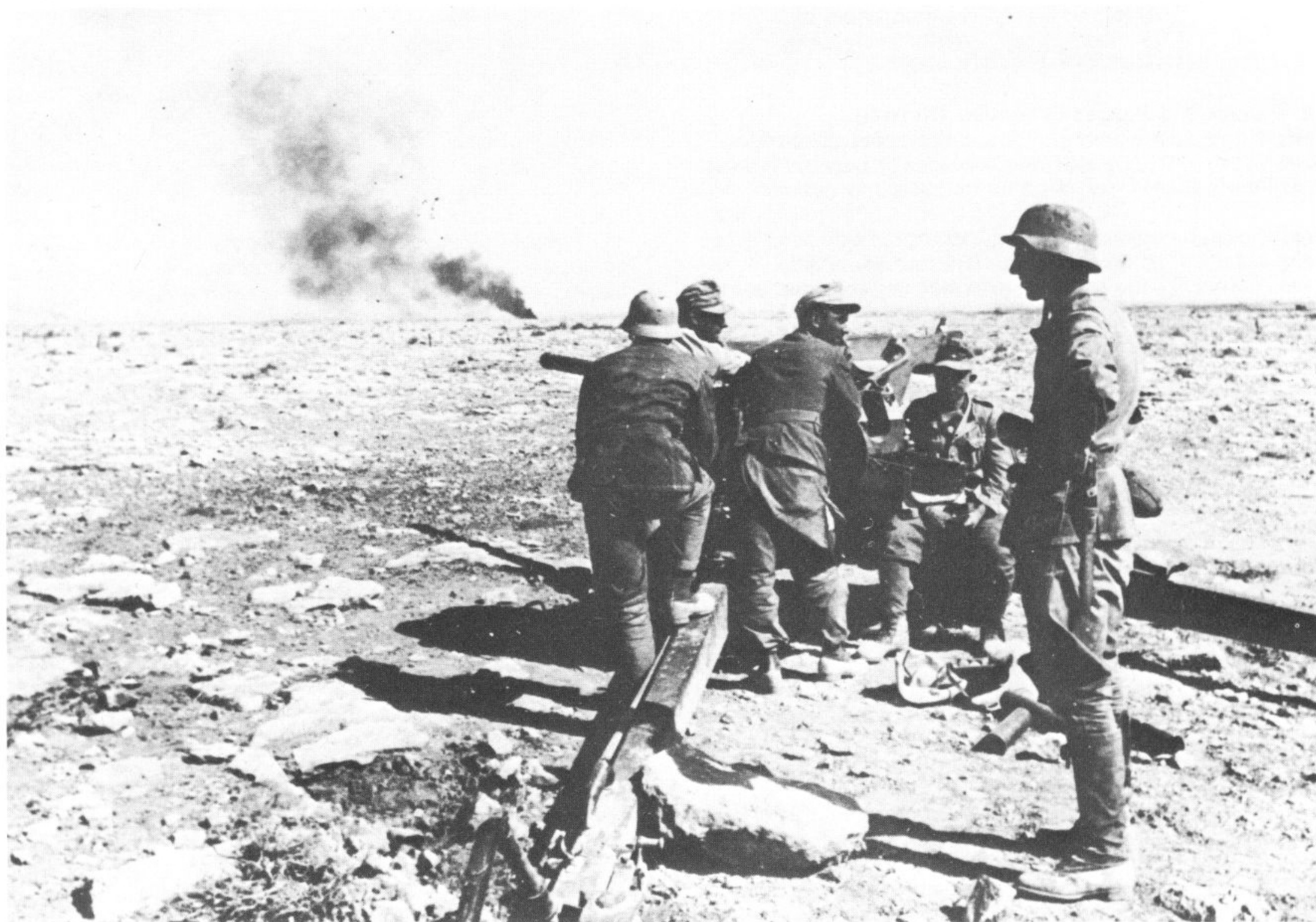
ABOVE: 5 cm Pak 38 engaging tanks on the Eastern Front. The loader – positioned to the left of the gun breech – has a leather sling with a swivel fitted across his shoulder which is used for manhandling the piece when changing deployments. A tank which the gun has just hit is in the background directly above the gun commander's hand. This Pak 38 with its low silhouette was probably invisible – even in the open countryside shown here – to the closed down Soviet tanks.
