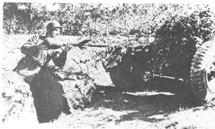
Pak 35/36 with the 3.7 cm Stielgranate 41. This was a hollow charge spigot grenade.
