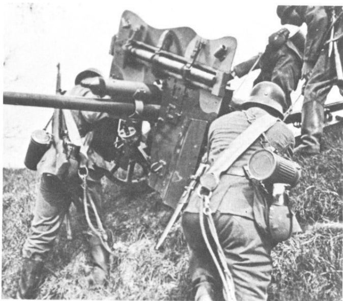
Pak 35/36 with the 3.7 cm Stielgranate 41. This was a hollow charge spigot grenade.
