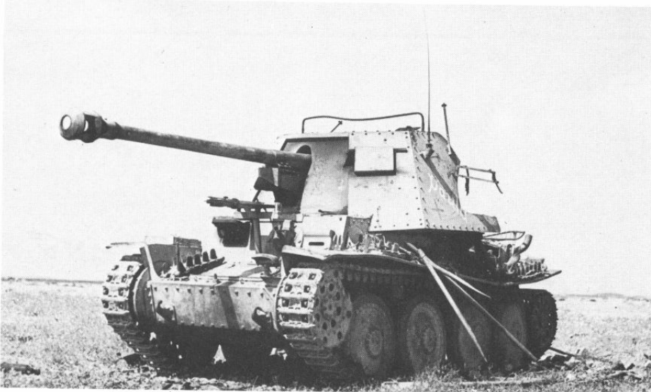
The Marder III Ausf H SdKfz 139 mounted the 7.5 cm Pak 40 on a virtually unmodified PzKpfw 38(t) chassis which even retained the bow machine gun of the tank.
