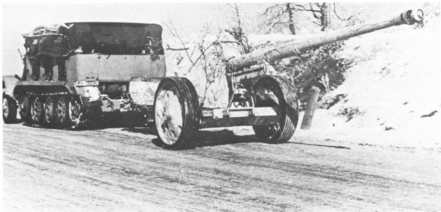
ABOVE: An 8.8 cm Pak 43/41 L71 under tow by a SdKfz 6.5 tonne prime mover. The barrel has been wound with wire to hold foliage as camouflage.
