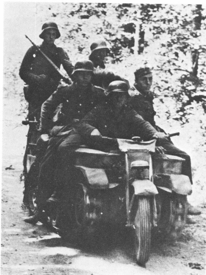
Overloaded NSU Kettenrad which could be used to tow light guns.
